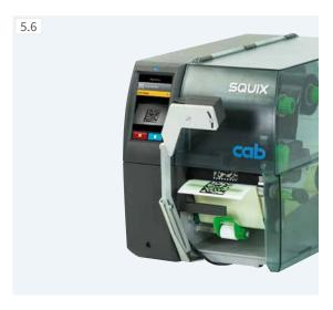
**CC200-SQ scanner** for detecting linear 1D barcodes, 2D and stacked codes A camera checks a code printed on a label in horizontal or vertical direction in terms of legibility or content. In the case of a bad coding, printing stops and the label can be removed by hand. Retracting such labels after stopping and blackening them is another printer option.
