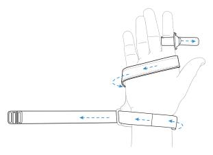
4. Fasten the strap on the index finger. Continue to tighten the strap around the wrist.
