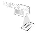
**Note:** If the light level in the room is not high enough, the barcode may not be read. If room lighting is not sufficient, auxiliary lighting may improve scanning performance
