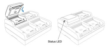
It is important that batteries are inserted into the charging pocket correctly. Inserting the battery incorrectly could result in damage to the battery or the charger.
