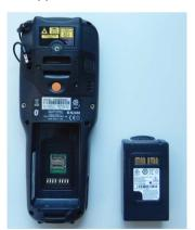
4. Insert the new battery pack into the slot (see Install the Battery on page 17).
