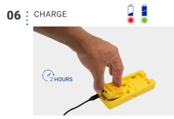
The pins face down. Insert the HandScanner in the Datalogic Charging Station.
