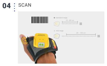
Press the textile trigger. Aim at the barcode and scan.
