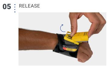
Use your fingers to press between HandScanner and the fastening rail of the Hand Trigger. Press the HandScanner up slightly and push it forward without scratching over the pins.
