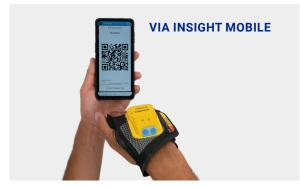
Open the app symbol "Insight Mobile" on the mobile device and scan the Pairing Barcode. To download the app and configure the device, register at https://www.datalogic.com/handscanner/config.
