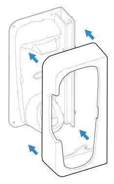
11. Secure the bezel cover in place with the four (4) M2.5 screws supplied.
