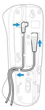
8. Lower the two (2) key holes on the base over the two (2) screw heads on the L-bracket. Slide base toward the bottom edge of the L-bracket and into the key hole channel locks.
