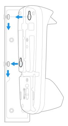
9. Secure the charge base to the L-bracket with two (2) M4 screws supplied. Do not skip this step or cradle movement under the bezel cover may occur.
