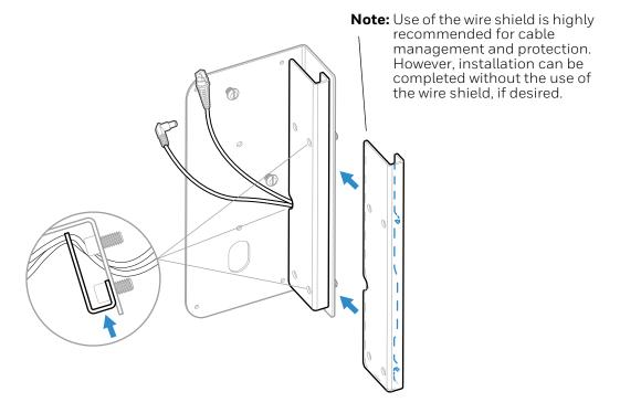
7. Attach the power and communication cable to the base. Arrange the wires so they exit out the side indicated below.
