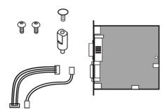
The only tools required for installation are the #T10 and #T20 Torx screwdrivers.
