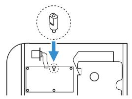
9. Insert the Applicator Interface Board into the printer and secure the board assembly to the printer with two torx screws.
