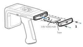
To uninstall the battery, remove the battery cover screws and then the battery cover. Pull the tape on the battery to pull the battery out.
