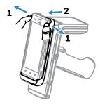
5. Unload the bracket: hold the handle with one hand and lift it from the side of the bracket with other hand.
