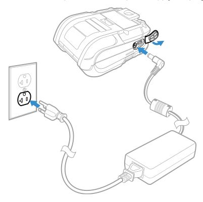
**Note:** Operating the printer while it is connected to the AC power supply can shorten the life of the battery and is not recommended.
