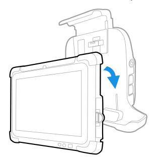
**Note:** The slot on the back of the tablet (A) must align with the tab on the front of the dock (B).
