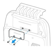
4. Align the slot on the push release latch with the latch support, then attach the push release latch using the M2.5  $\times$  5 round head screws.
