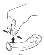
2. Remove the battery and end cap.
