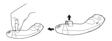
2. Remove the battery and end cap.
