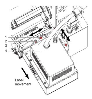
Fig. 5 Adjusting the air-jet module sidewise
