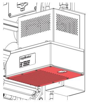
Fig. 12 Cleaning the suction plate
