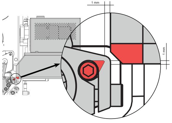
Fig. 7 Adjusting the height of the air-jet module
