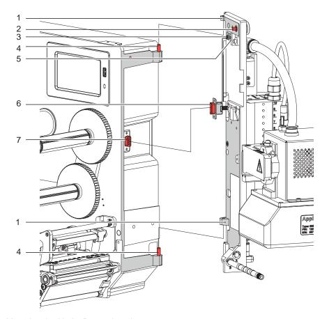
Fig. 4 Mounting the Air-Jet Box to the printer
