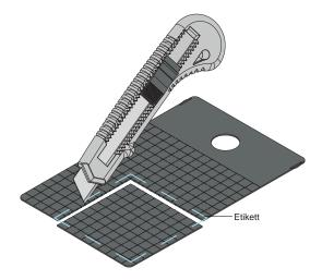
Fig. 14 Cutting the aperture
