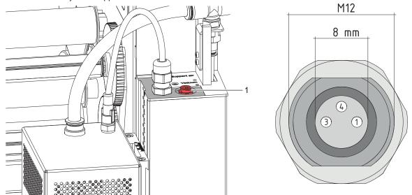
Fig. 10 Start signal connector on the applicator
