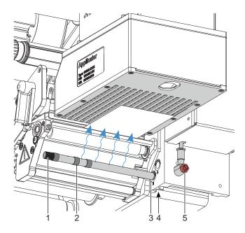
Fig. 9 Adjust the blow tube
