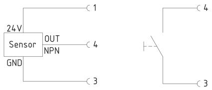
Fig. 11 Examples of connections of start sensors
