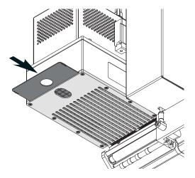
Fig. 15 Slide in the former plate
