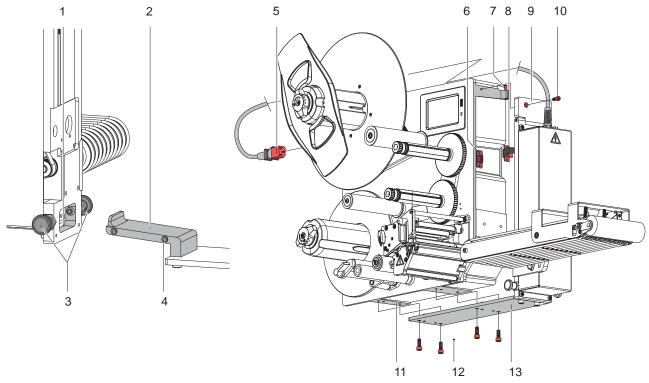
Fig. 7 Mounting and dismounting the applicator
