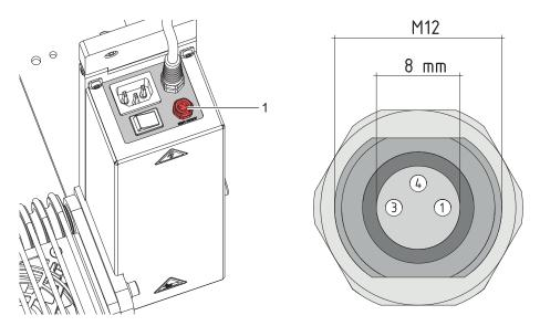
Fig. 8 Start signal connector on the applicator
