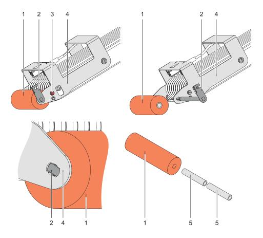
Fig. 13 Exchanging the pinch roller
