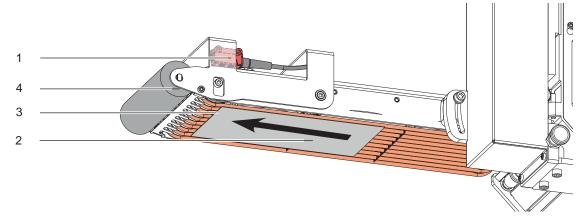
Fig. 11 Label transport/reflex sensor
