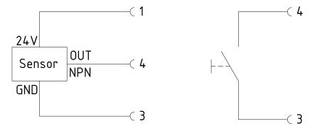
Fig. 9 Examples of connections of start sensors
