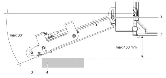
Fig. 10 Angle of the applicator to the printer
