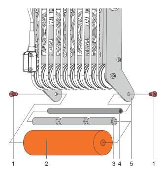
Fig. 13 Exchanging the pinch roller
