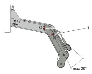
Fig. 10 Angle of the applicator to the printer
