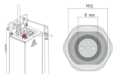
Fig. 8 Start signal connector on the applicator
