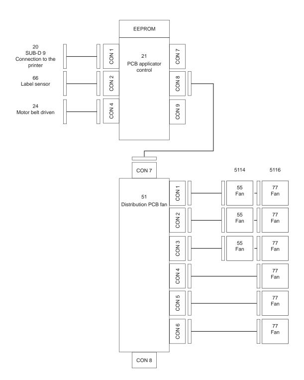
Fig. 14 Block diagram
