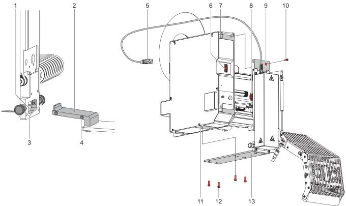
Fig. 7 Mounting and dismounting the applicator
