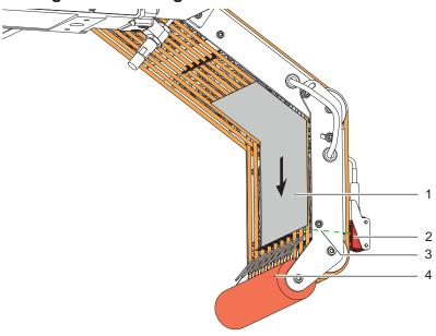
Fig. 11 Label transport/reflex sensor
