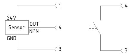
Fig. 9 Examples of connections of start sensors
