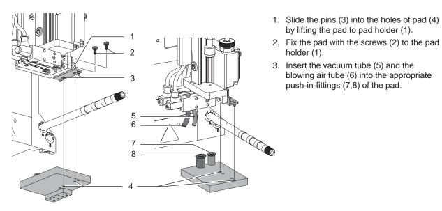
Fig. 11 Mounting the pad
