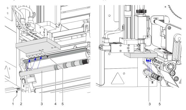
Fig. 22 Adjust the blow tube
