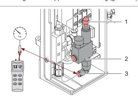
Fig. 32 Pressure reduction valve cylinder Z
