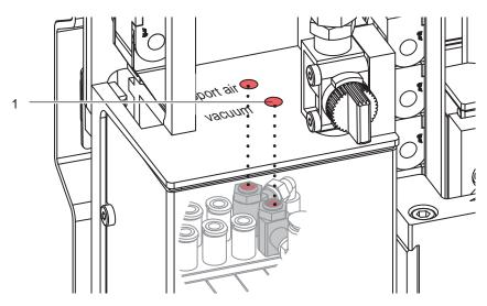
Fig. 20 Throttle valve "vacuum"
