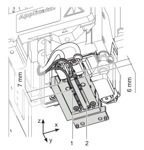
Fig. 34 Sensors on cylinder Y
