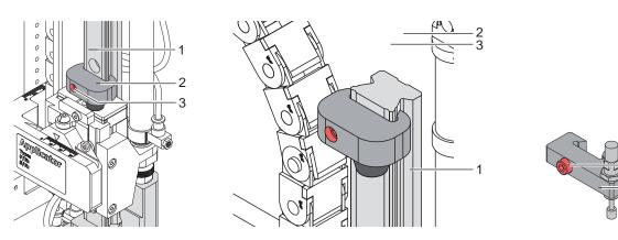
Fig. 9 Stopper as transport lock
