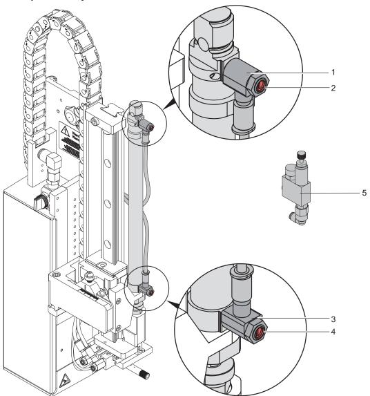
Fig. 26 Throttle valves on the cylinder Z
