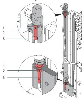
Fig. 27 Sensors on cylinder Z
