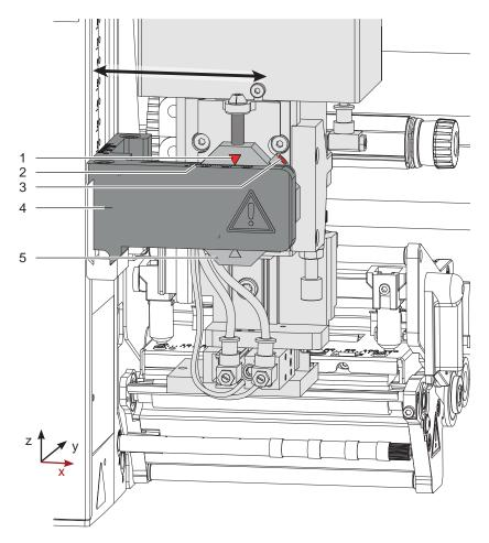
Fig. 17 Displacement in the Y direction
