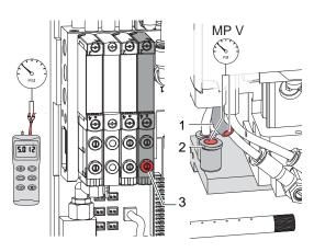
Use a manometer with a measurement area -7 to 7 bar for measurement the pressure.
