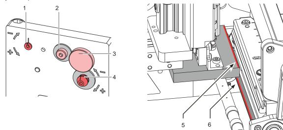
Fig. 14 Aligning the pad to the dispensing plate
