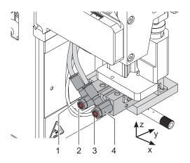
Fig. 33 One-way flow control valve on cylinder Y
