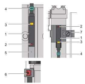
Fig. 19 Sensor / Mounting
