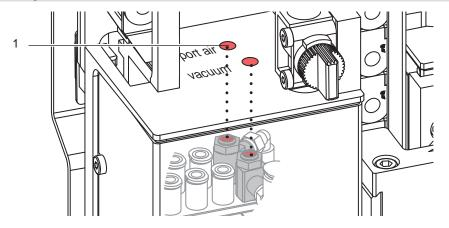
Fig. 23 Throttle valve "support air"
