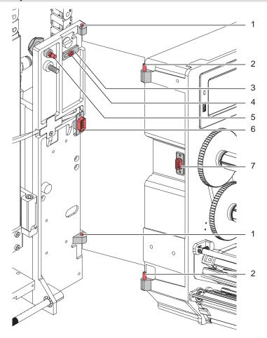
Fig. 7 Mounting applicator to printer
