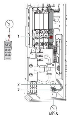
Use a manometer with a measurement range of -7 to 7 bar to control the pressure.
