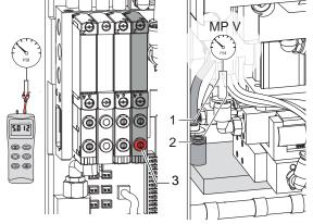
Use a manometer with a measurement range of -7 to 7 bar
