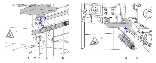
Fig. 21 Adjust the blow tube
