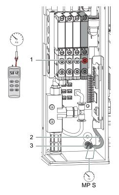
Use a manometer with a measurement area -7 to 7 bar for measurement the pressure.
