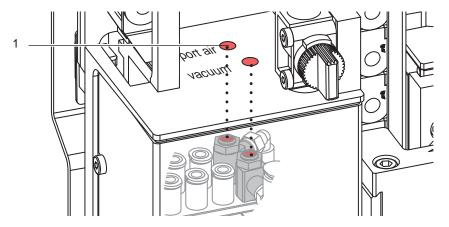
Fig. 22 Throttle valve "support air"
