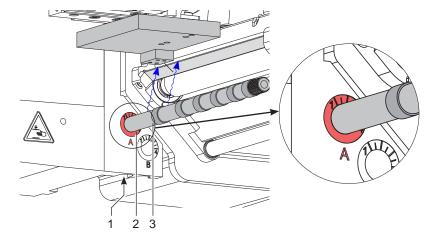
Fig. 12 Mounting the blow tube
