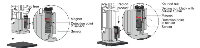
Fig. 28 Labelling sensor principle
