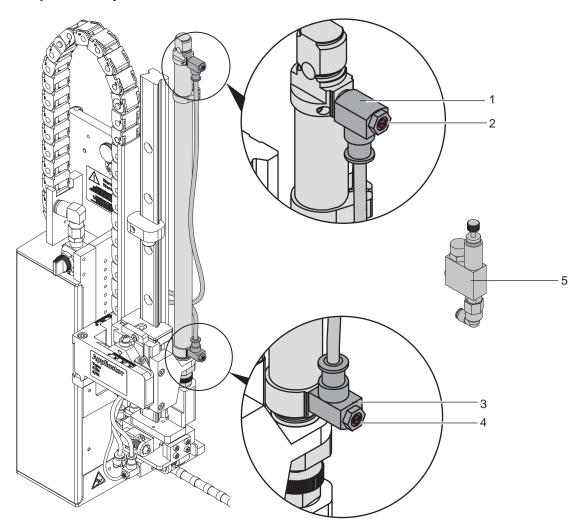
Fig. 26 Throttle valves on the cylinder Z
