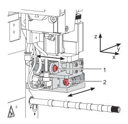
Fig. 24 Adjusting the labeling position
