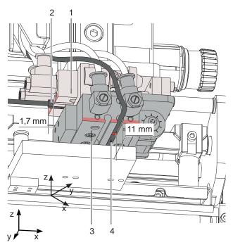
Fig. 34 Sensors on cylinder X/Y
