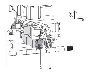
Fig. 33 One-Way Flow Control Valve on Cylinder X/Y
