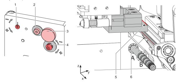
Fig. 13 Aligning the pad to the dispensing plate
