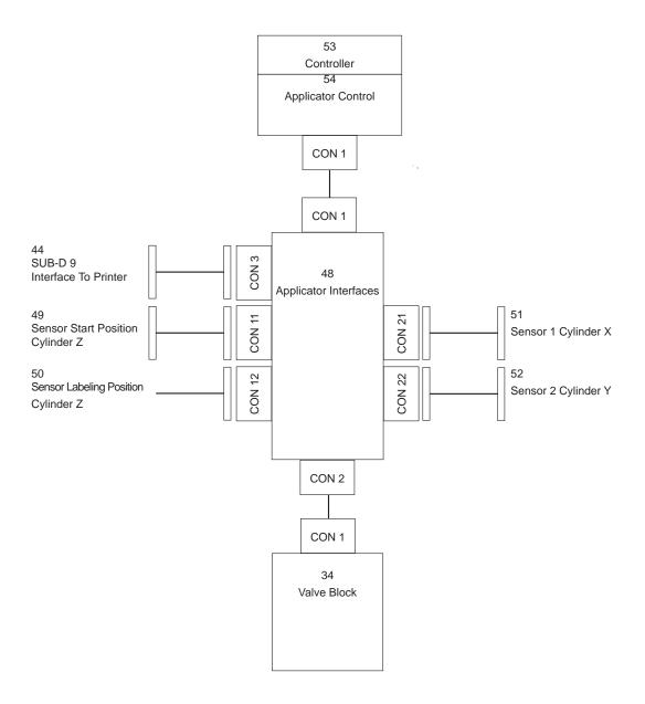
Fig. 39 Block diagram 4414
