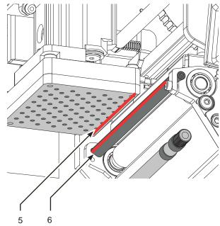
Fig. 14 Aligning the pad to the dispensing plate
