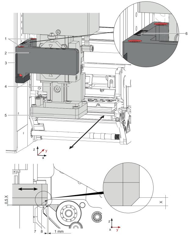
Fig. 15 Displacement in the Y direction
