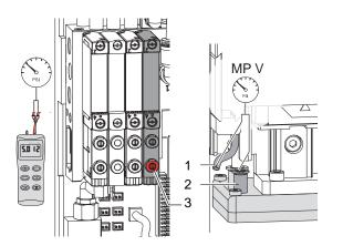
Fig. 19 Measuring points for the vacuum
