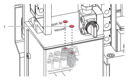
Fig. 18 Throttle valve "vacuum"
