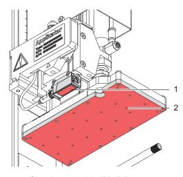
Fig. 6 Cleaning pad with slide foil
