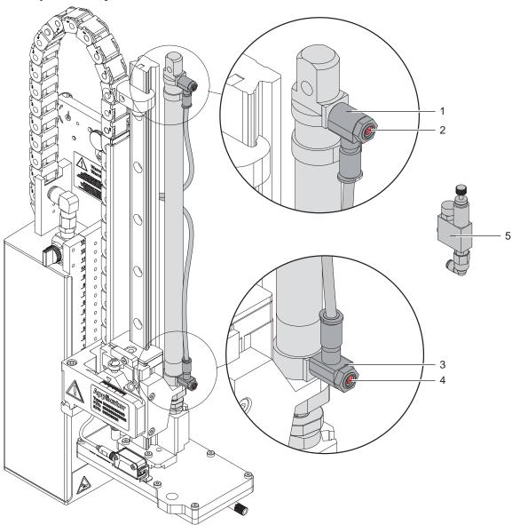
Fig. 25 Throttle valves of cylinder Z
