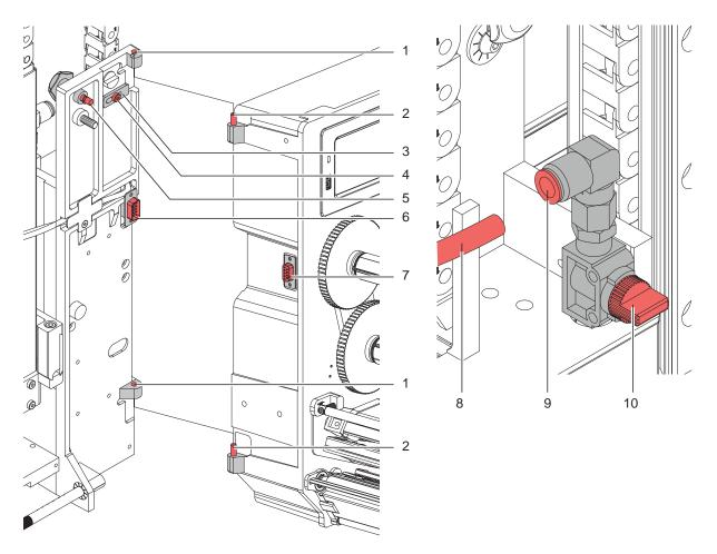
Fig. 10 Mounting applicator on printer
