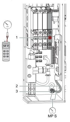
Fig. 22 Measuring points to measure the support air
