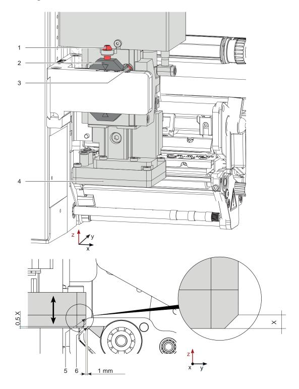
Fig. 16 Displacement in the Z direction
