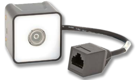
The HF520 is a self-contained unit that includes decoded 2D optics, housing, exit window, and a TTL-RS232 interface board.
