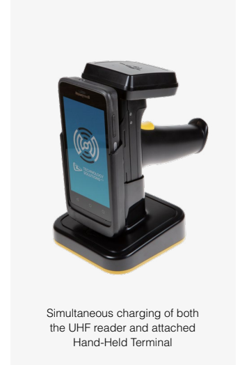
Integrated ePop-Loq socket allows data and charge connections to a Smartphone or Hand-Held Terminal
