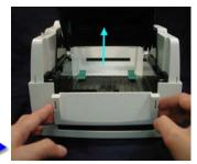
Plug in the connector according to photo shown. (3 pin onto converting board).
