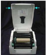
Loosen and then lift the upper print mechanism by pressing the locking tenons.
