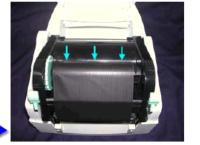
**Note:** Before loading a new transfer ribbon roll, we recommend to clean the printhead with printhead and roll cleaner (97.20.002).
