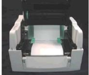
Close the upper print mechanism from the top to finish label installation.
