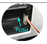
Clip in the right side of the cutter module first and then secure the left side.
