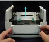
Open the mechanism by pressing the locking tenon, plug in the cable connector of the cutter module onto the switch board socket.
