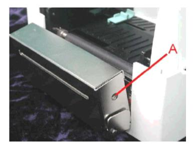
A cutter adjusting hole is present on both sides (where A is pointing to).
